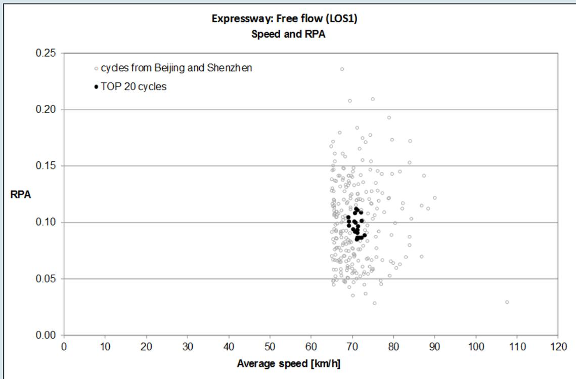
**Figure 9: Selected top 20 cycles for passenger cars based on average speed, RPA and stop time (not included in the figure) using the example of the traffic situation “Expressway”: free flow.**
